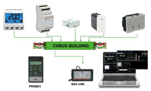
Or by means of an Ethernet connection to the system supervisor. Also with Wi-Fi...
