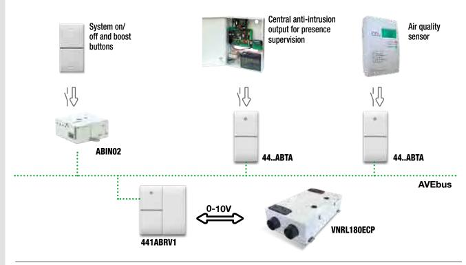
Decentralised CMV with "SOLAIR" heat recovery - Control with cod. 44..AB-IRT
