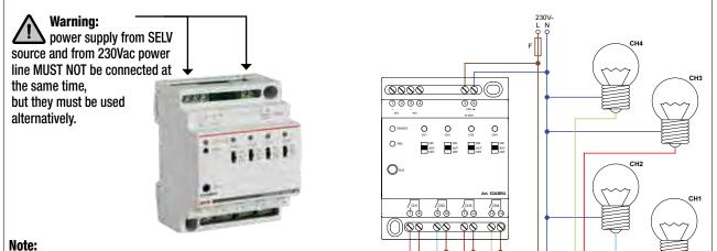
the micro-two-way switches placed on the front, if in the ON or OFF position, manually force the output, while in the AUTO position the output follows the controls received from the bus.
