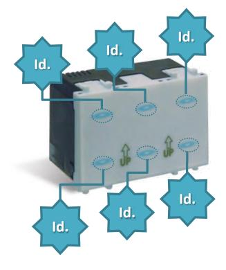
The address of each channel of the device is made up of two hexadecimal alphanumeric characters:
