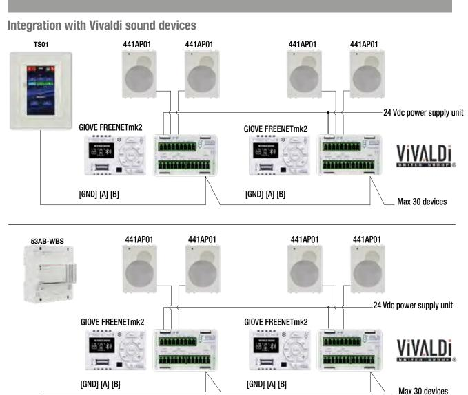
Functions: ON, OFF - Volume Control and MUTE - High and Low tone control - Source change TUNER, USB, AUX-IN, B.T. and MIC - Change of radio station frequency (+/- 0.1Hz) - Change of USB folder and MP3 File.
