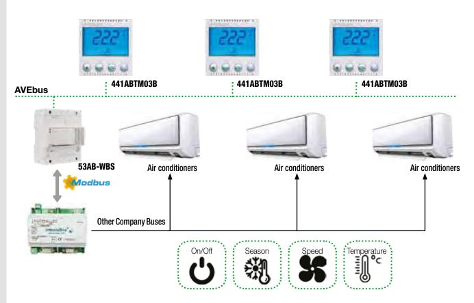
The DOMINAplus supervisors range interfaces with the leading brands used for Central Air Conditioning by using the Modbus standard protocol.
