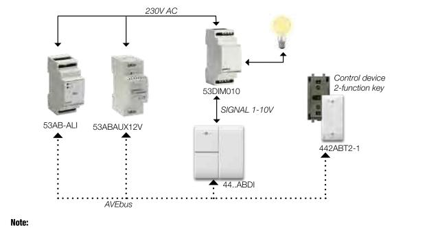
Instead of the common lamp, the device is able to control LED strips by simply installing an electronic controller for LED and/or LED RGB, instead of item cod. 53DIM010. For information about the compatibility of these controllers, please contact AVE's sales network or Technical Assistance Service
