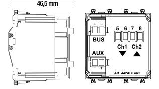
IP41 if completed with keys and installed in the corresponding flush-mounted box.
