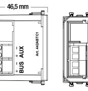
1 m. "hidden" S.44 (22.5 w x 45 h x 46.5 d) mm, to complete with front plate.
