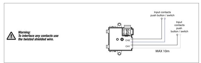
2-channel hidden contact interface - dimensions (WxHxD) 54x41x18 mm
