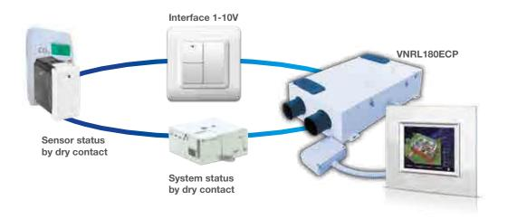
Moreover, with the analogue interface DOMINAplus acquires signals from the air quality sensors and, if necessary, sends the command via the infra-red interface device to manage the single flow ventilation unit alternated with heat recovery, all under optional supervision from the Touch screen.
